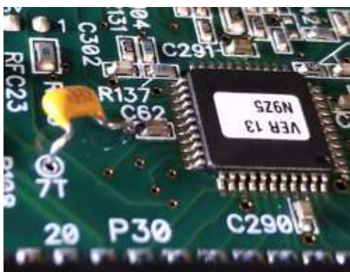
Figure 9: l/h: Disconnected Elecraft-installed cap in 11369, r/h: oscillation present
