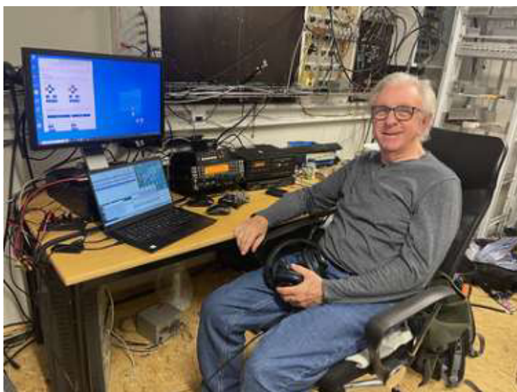
George, TF/K5KG at Station B: K3 and KPA500 amp. Antenna matrix on back wall.
