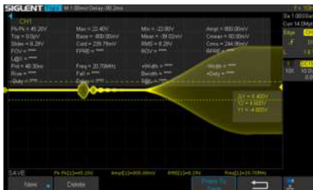
Figure 9: l/h: Disconnected Elecraft-installed cap in 11369, r/h: oscillation present
