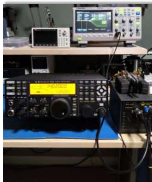
Figure 1: Measurement setup: K3S attached to a 50Ω load with signal tap
