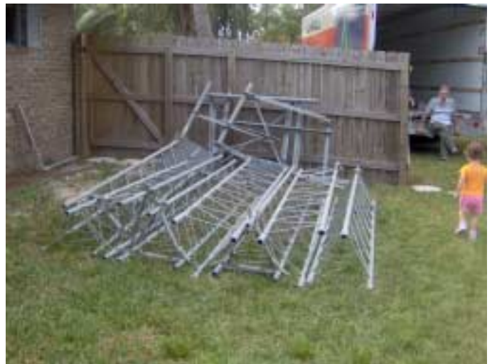
Here are pictures after the unload. 340 feet of Rohn 55G with plenty of accessories
