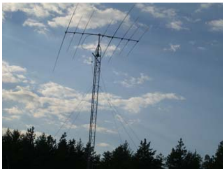
20/15/10 m Cycle 24 TX-38 Tribander on a 40 ft tower was standard equipment at all sites. This one was at N1S.
