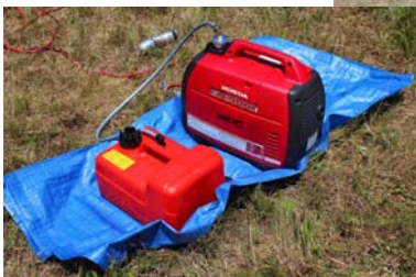
A 2 KW Power Generator was provided at each site.
