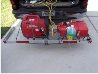
2 KW power plant
