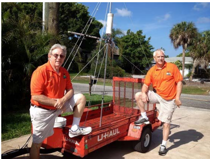
Above - The K4KG/M setup features a vertical antenna mounted on a trailer behind their vehicle. L-R - George and Jim have used this setup for the last several FQPs very effectively.
