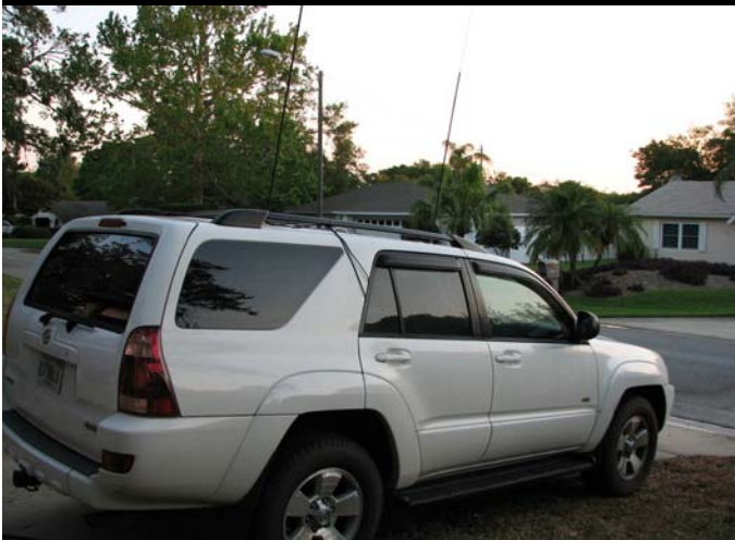
Above: N4EEB's Toyota 4-Runner with 20 meter (fore) and 40 meter( aft) hamsticks.
