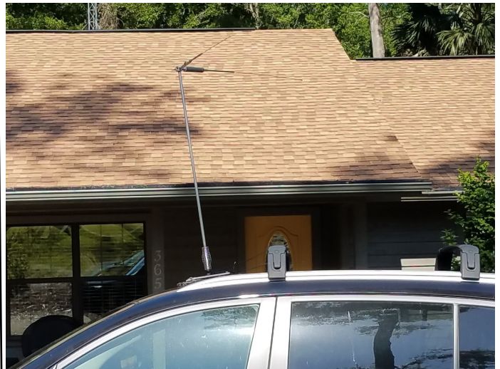
N4FP 2016 Kia Sportage with horizontally mounted 20 and 40 meter Hustler resonators. An unusual antenna, but Wayne says it works very well. He has been using it for the past five years, earlier on a different vehicle.
