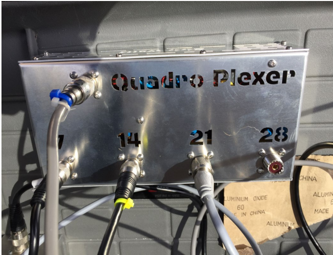
Quadriplexer experiment to reduce RFI
