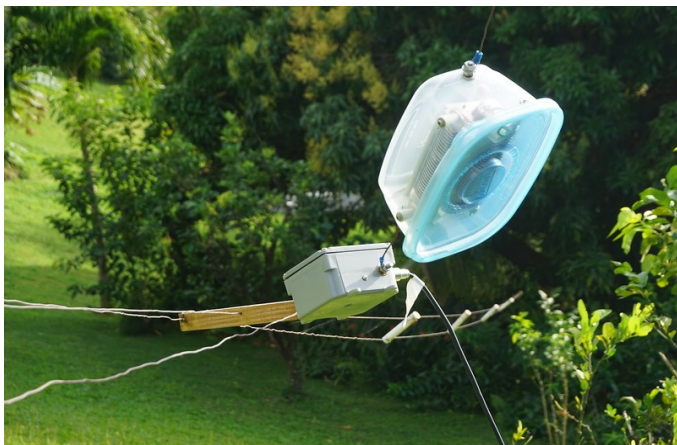
Matching Unit for 160 Meter Folded Counterpoise
