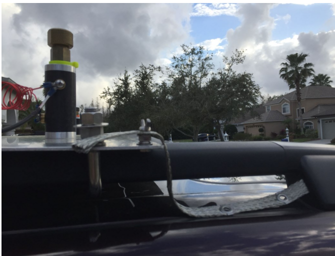
NX4N - New antenna plate to roof grounding strap ( 1 of 4 straps)
