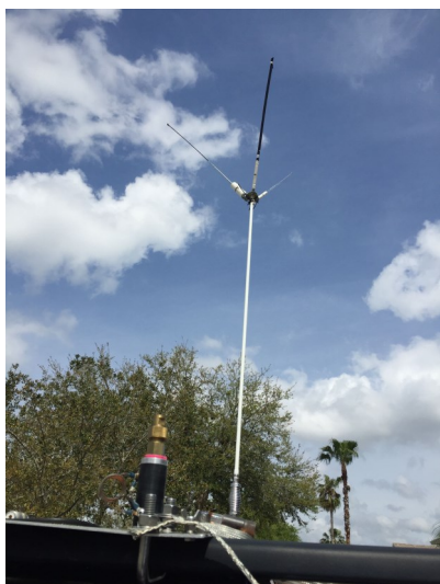
K4OJ MM Mobile - Single Multi-band Antenna for quadruplexer RFI experiment.
