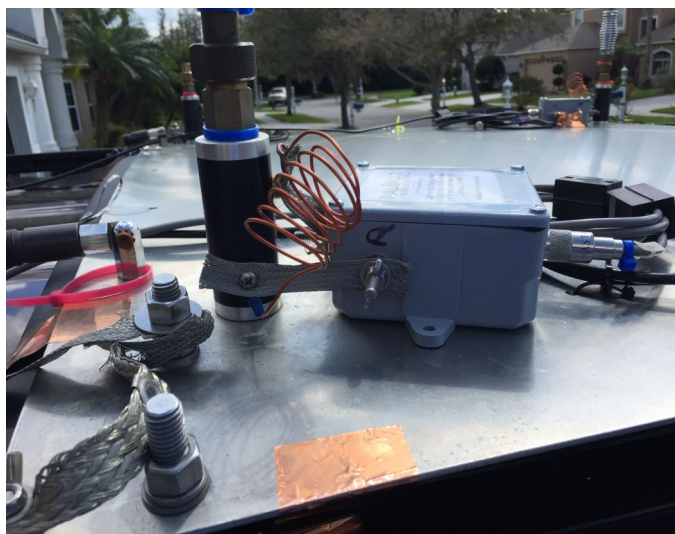
Closeup of feedpoint RFI mitigation (lots going on if you look closely!)
