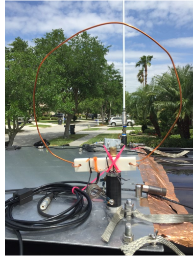
RF Loop antenna to fight RFI
