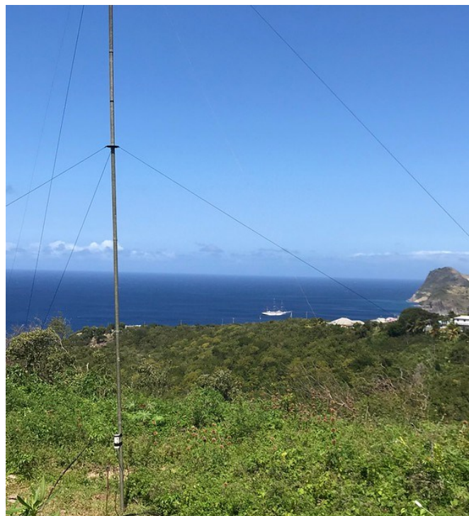
Fiberglass Pole supporting a K9AY Rx Loop
