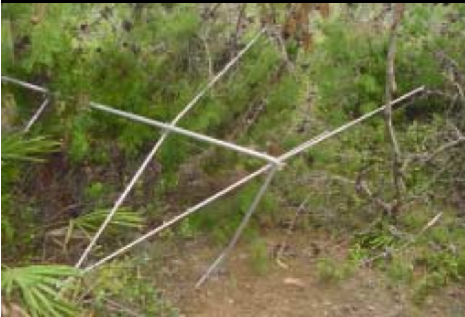
K4LQ's 6 Meter beam after cutting away most of the pine trees that had fallen on it.
