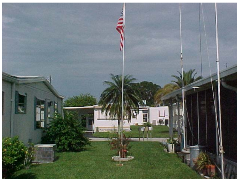
FCGer George N3ISH operates this flagpole antenna with good results on 60, 40, 30 and 20 meters from his Naples QTH. Switching in the formidable looking coil at the lower right puts it on 160 Meters.
