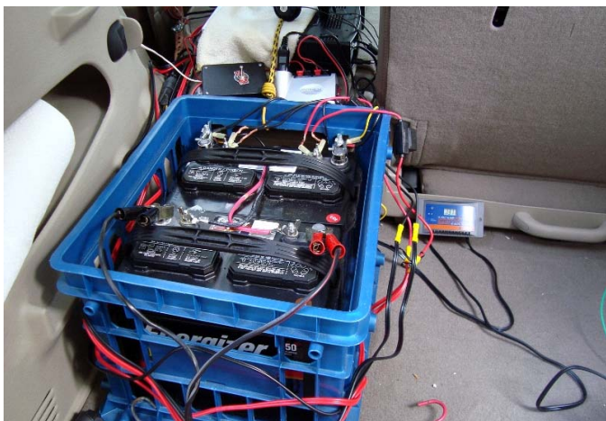
Above: MFJ Tuner + one of those newfangled keying devices (not used). Below - The deep cycle battery configuration that powered the whole operation.
