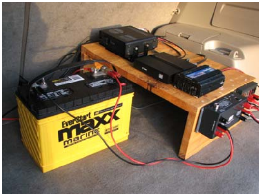
Equipment deck in the cargo area of the 4-Runner. Icom IC-7000, LDG AT7000 Tuner, MFJ Boost Regulator, AC inverter, RigRunner
