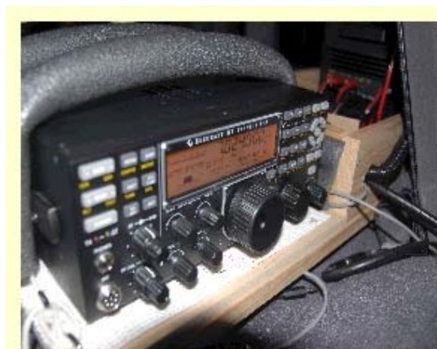
The Elecraft K-3 transceiver is tied down in the rear compartment and controlled by a K-3 remote that Chuck has developed for CQ/X
